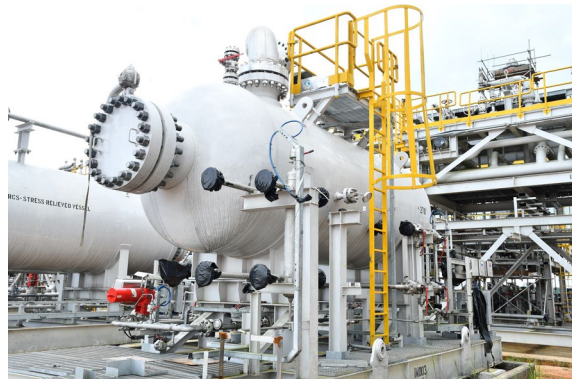
GAS FEED COOLER OUTLET SEPARATOR
